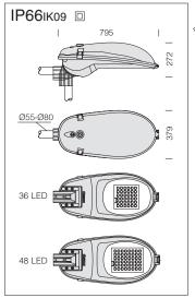
**LED:** Power factor ≥0.9. Luminous flux maintenance 80%: >100.000h (L80B10).
